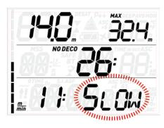
If the ascent rate exceeds 12m/min / 40ft/min at a depth below 12m / 40ft, # blinks as well. If a speed in excess of 12m/min / 40ft/min is maintained for two thirds or more of the depth at which the alarm was first triggered, Quad considers it a dive violation and the display will show the steady # .
