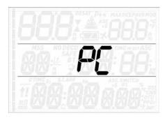
This submenu allows you to download your dive data to a PC or Mac. Press the **ENTER** button and the display will show **PC ready**, symbolizing that Quad is ready to communicate.
