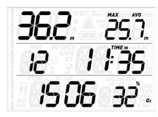
Press **ENTER** to view the next page of the dive log, which shows the surface interval prior to the dive alternating with the dive time and **CNS** (alternating between start and end value) in the bottom row. In case more than one gas was used in the dive, information about **G2** and **G3** if applicable is shown alternating with G1 on the first page.
