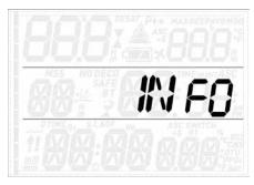
This submenu provides information about the hardware and software of your Quad and about the status of the battery: **OK** means the battery is good, **LOW** means the battery is weak but you can still do a few more dives, and **KO** means the battery is very low and Quad won't function as a dive computer.
