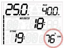
When the oxygen toxicity level approaches 100% the alarm is repeated for 5 seconds in one-minute intervals after the first occurrence and for as long as the value of CNS stays at or above 100%. Consider terminating the dive immediately!
