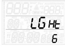
Quad has a backlight which can be activated in case of low ambient light. The backlight is activated by pressing and holding either of the upper buttons. During a dive, the backlight will stay on for the duration defined in this menu. You can choose between 1 and 10 seconds or you can set it to **on**. If you set it to **on**, the backlight will remain on until you press and hold either of the upper buttons again.
