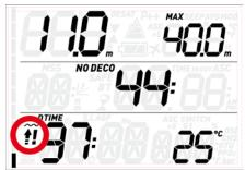
In this case, if the diver attempts a repetitive dive after surfacing, Quad will only function as a depth gauge and timer (bottom timer mode), and will display  $\P$  on the screen throughout the dive.
