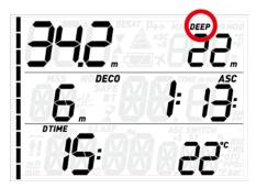
Upon reaching the optimum range for carrying out a deep stop (+/- 1m /3ft of the displayed depth), the deep stop itself will be shown in the top right corner with the label **DEEP** blinking, and a countdown timer appears to indicate the progress of the stop. Deep stops can be deactivated in a dedicated settings menu.
