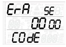
Quad allows you to reset the desaturation in the computer. Any tissue saturation information from a recent dive will be reset to zero and the computer treats the next dive as a non-repetitive dive. This is useful when the computer is loaned to another diver who has not dived in the last 24 hours.
