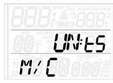
You can choose between metric (depth in meters, temperature in °C) and imperial units (depth in feet, temperature in °F).
