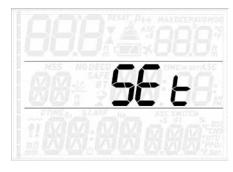
Quad's **SEt** menu allows you to change settings. Once inside this menu, press the **UP** or **DOWN** button to scroll between two submenus: **SEt dIVE**, where you can set parameters pertaining to the dive, and **SEt tIME**, where you can set parameters pertaining to time and date.
