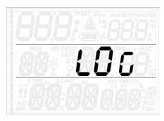
Quad can record the profiles of approximately 35 hours of diving, at a sampling rate of 5 seconds. The information can be transferred using the optional USB clip to PC via the Dive Organizer software or to a Mac via the Divers' Diary software. In addition, Quad can show most of the information directly on the display.
