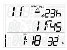
The other contains a condensed log of the last dive: maximum and average depth in the top row, dive time and set 02% in the bottom row. In addition, the bar graph shows the calculated nitrogen load in the leading tissue. You can use this to gauge your progress in getting rid of nitrogen as the surface interval grows. Quad continues to perform decompression-related calculations (nitrogen release), for as long as there is desaturation time left.
