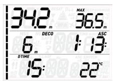
By pressing either of the upper buttons, you can modify the information displayed in the upper row. At each button press, the screen cycles through, max depth, average depth, MOD (nitrox only), deep stop (if activated and if calculated to be present), and an empty field.
